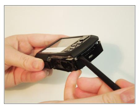
Pry off back outer casing using the black spudger or the blue prying tools
