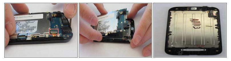
Pull back on the two circuit connections that attach to the main circuit board. Then remove the circuit board from behind the screen.
