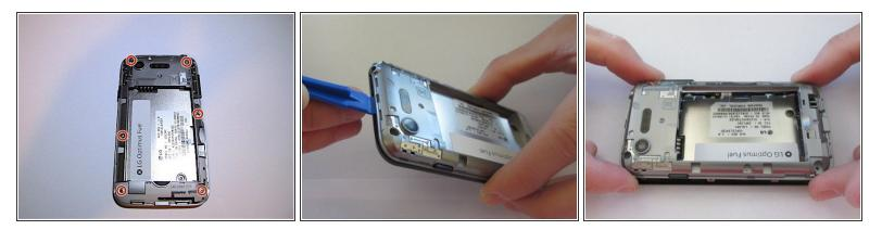
Remove the 6 screws using a size PH00 Phillips head screwdriver, and a plastic opening tool to fully remove the back panel.
