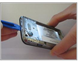
Remove the six 1.4mm screws using a Phillips head screwdriver with a size PH00 bit. Then fully remove the back panel with a plastic opening tool.
