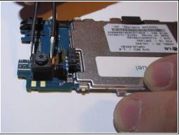
• The camera has been secured to the circuit board using an adhesive. Use a plastic opening tool and precision tweezers to remove it. Don't be afraid to use a little force when pulling at the camera.
