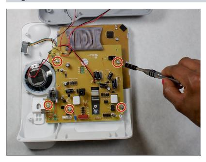
Use a bit driver to remove all five 5mm X 5mm Phillips head Motherboard screws.
