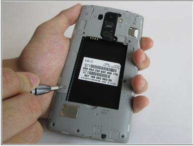
Carefully use the Phillips #00 screwdriver to remove the eleven 3.9mm visible screws found on the back. The screws to be removed are marked with the given indicators.
