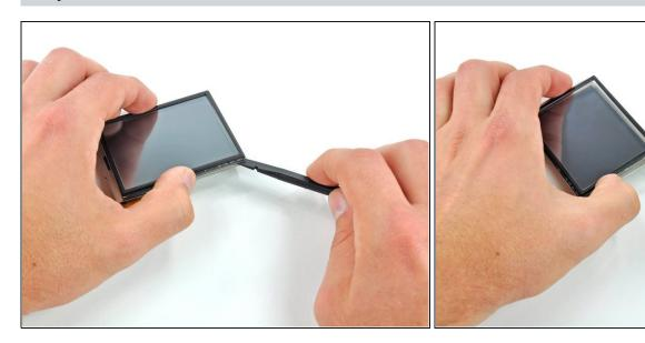
Repeat the above procedure for the remaining two corners to pry the touchscreen off the LCD frame.
