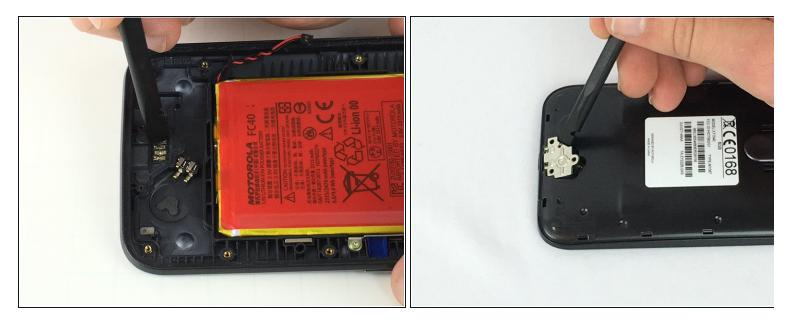
• Use a spudger to push out the charging port from the inside of the case and pry it off from the outside of the case.
