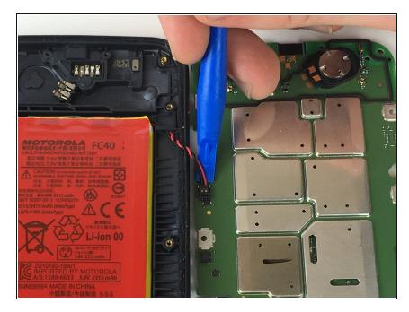
• Use a plastic opening tool to disconnect the battery wires from the motherboard.
