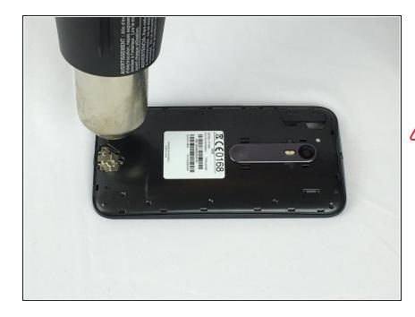
If the charging port is secured with adhesive, use a heat gun around the charging port for ten seconds to loosen the adhesive.
