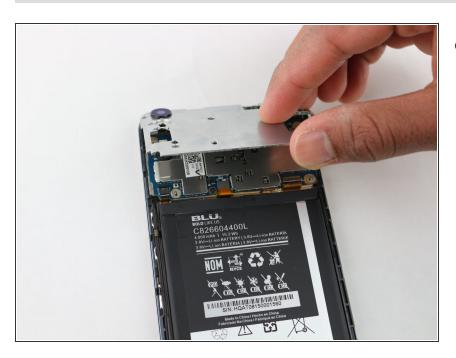
After all the screws are out, lift the protective metal cover off of the phone. Lift from the bottom of the cover.
