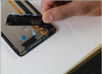
Lift the module where the speaker is located.
