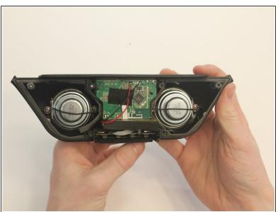
Slide off the inner cover. It pulls apart and is held on by a small amount of glue.
