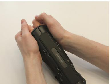
From the same side you just unscrewed, use a plastic opening tool to unwedge the inner cover on both sides of the base.
