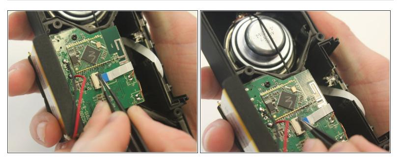
Undo the connector of the flat white ribbon between the switches and the logic board.
