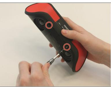
Using a <u>Phillips PH0 3 mm-bit screwdriver</u>, remove the six screws on the inner layer of the Taco.
