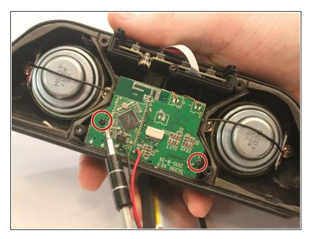
Undo the two black 3mm screws on the logic board using the PH0 screwdriver.
