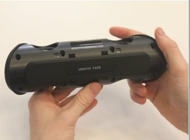
Repeat the previous step on the opposite side to remove the other outer casing.
