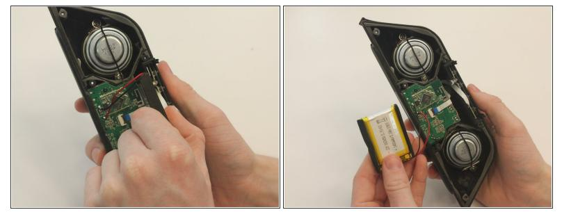
Move the battery out of the way of the connector.
