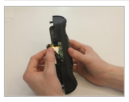
Remove the rubber covering from the buttons.
