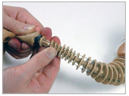
• There is a dab of glue at the tip of the tail. The articulated tail is capable of a surprising variety of movement.
