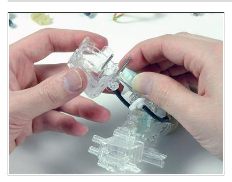
The tail has four wires, and each pair is connected at a gear. One motor can move the tail from side to side and the other moves it up and down. Combining these two movements in varying proportions gives the tail an amazingly flexible range of motion.
