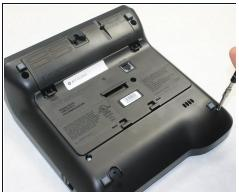
• Remove five 9.5 mm Phillips #1 screws from the back panel of the phone.
