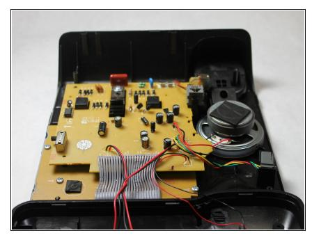
⚠ When setting the back panel down, be careful to not rip any of the wires off of the internal components.
