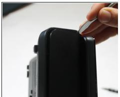
Slide the metal spudger into the crack and continue around to the front panel of the phone.
