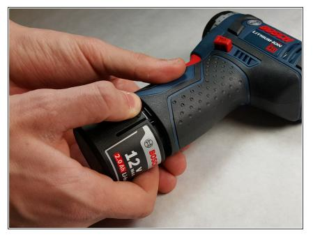
Pinch the two release tabs on the sides of the battery, and slide the battery out.
