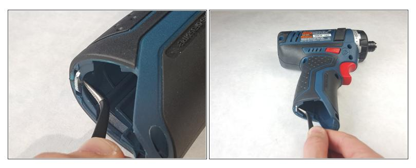
• Locate the clip that binds the two halves of the outer casing together on the rear edge of the battery shaft. Remove the clip with the angled tweezers.
