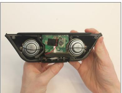
Slide off the inner cover. It pulls apart and is held on by a small amount of glue.
