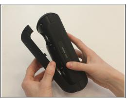
Starting with the Taco on its side, use the plastic opening tool to pop off the outer casing near the base.
