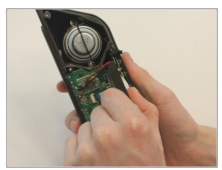
Remove the battery from the side of the casing.
