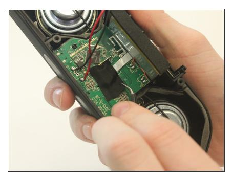
A black fabric covers the ribbon retaining flap, remove it using the curved tweezers as it can be a fire hazard when soldering.
