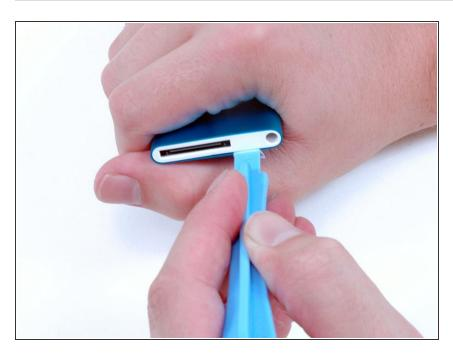
Pry the bottom bezel off using the same technique as the top.
