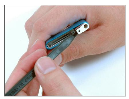
Pry out the headphone jack slowly with a spudger. Do not remove the headphone jack entirely, as it is connected via a fragile ribbon connector to the click wheel.
