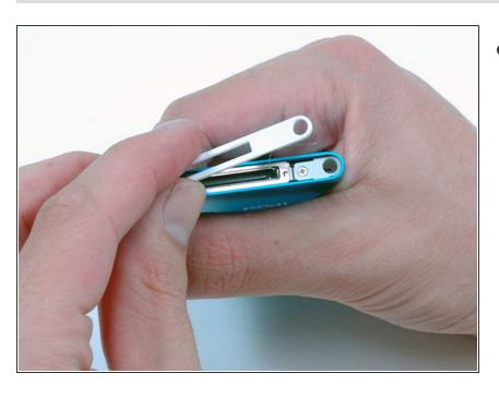
Lift the bottom bezel off. It's glued on using a mild adhesive, so some force may be required.
