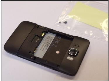
• Remove the four black 3.5mm T5 screws from the back of the phone.
