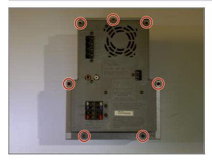
Remove these seven 11.5 mm screws and place aside.
