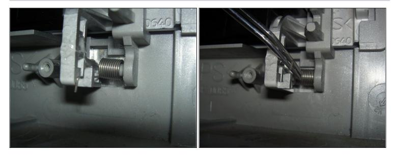
• Remove the spring from its slot using tweezers.
