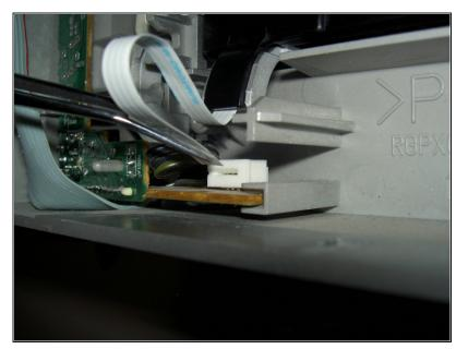
Using tweezers or fingers, pull firmly on the base of this cord until it pops out of its slot.
