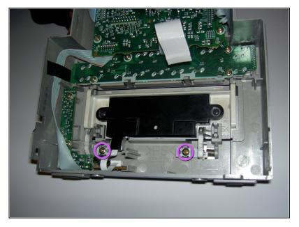
Remove the two 11.5 mm screws indicated and set aside in a safe place.
