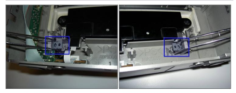
• Using <u>tweezers</u>, remove the two restraints indicated and place with the screws removed in the previous step.
