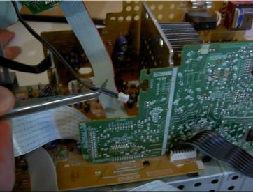
Disconnect the black wire by gripping the wire at the base and pulling gently until released.
