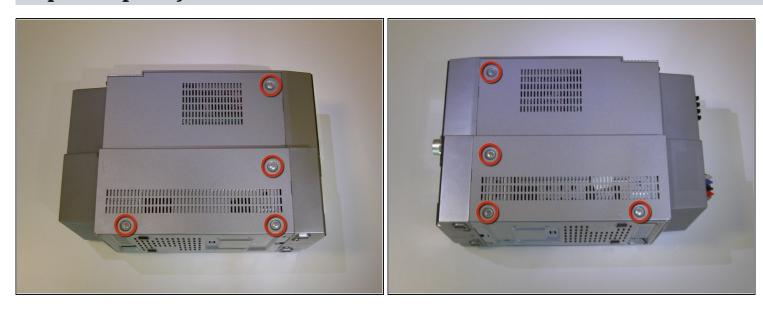
• With a Phillips #0 screwdriver, remove the eight 9.5mm screws attached to the left and right panels of the device.
