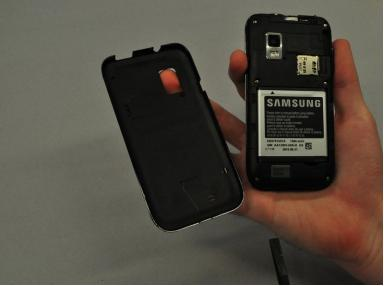
Insert the edge of the spudger into the slit and use it to pry the back case off of the phone.
