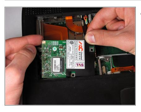
Using your fingers, lift the modem from the socket it is plugged into.
