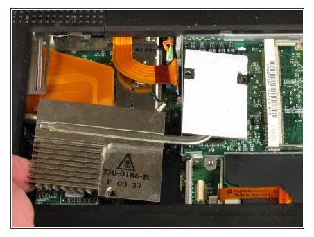
Lift up the heat sink unit from the left side and remove.
