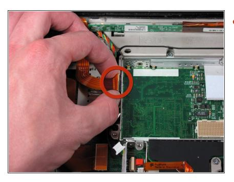
Disconnect the display cable from the logic board.
