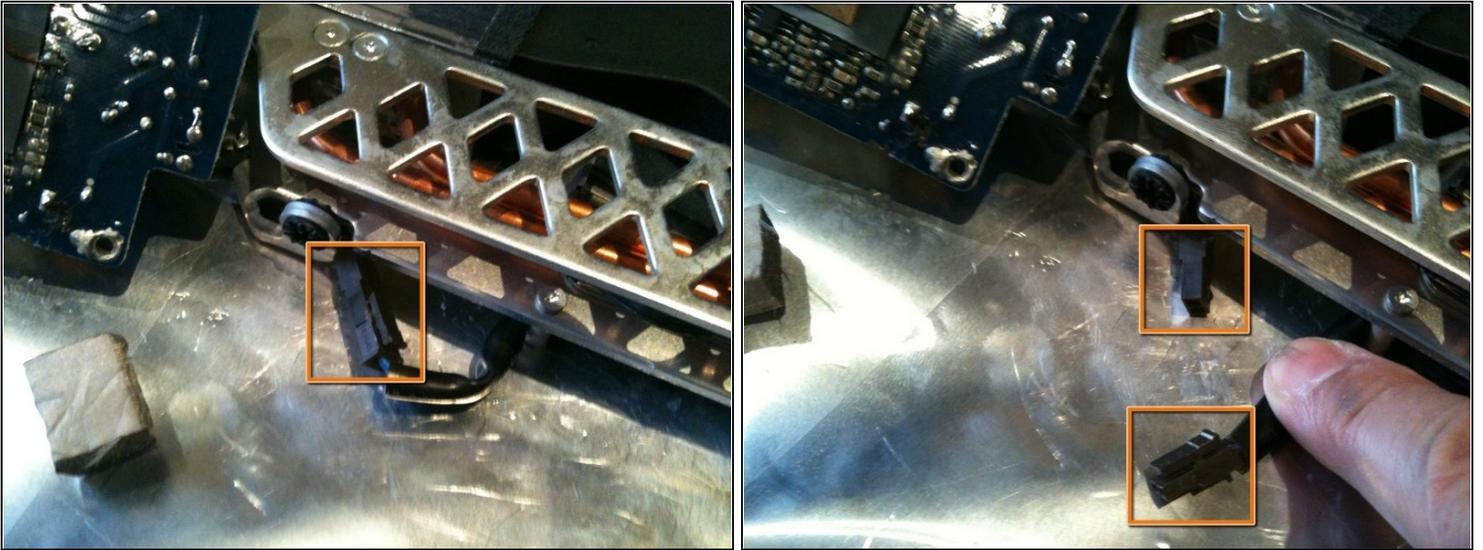
**⚠** Disconnect the right side connector (output) on the power supply and Gently pull the power supply out while feeding the connector under the metal bracket
