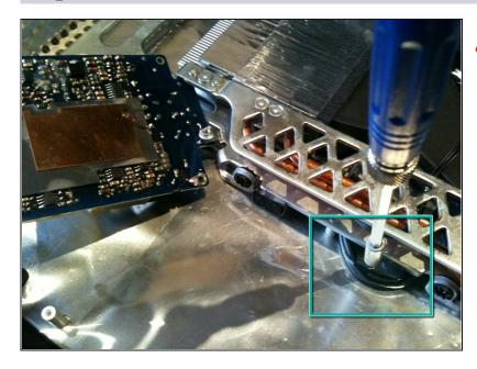
▲ Locate the black cable that runs from the right side (input) of the powers supply under the metal frame. Using a rounded (not sharp) tool gently bring the cable out from under the metal frame
