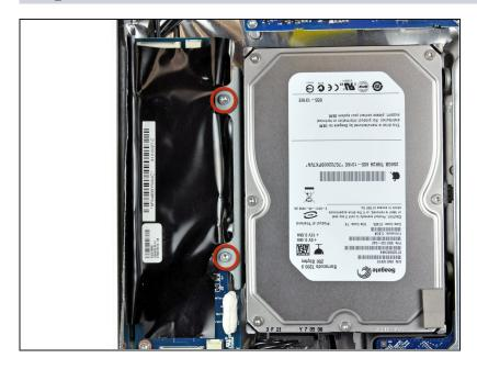
Remove the two 9.2 mm T10 Torx screws securing the hard drive bracket to the rear case.
