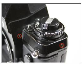
Use 00 Phillips head screwdriver to remove the screws from the top case (6 in all).
