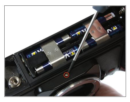
Use 00 Phillips head screwdriver to remove the screw from the bottom of the front black case.
