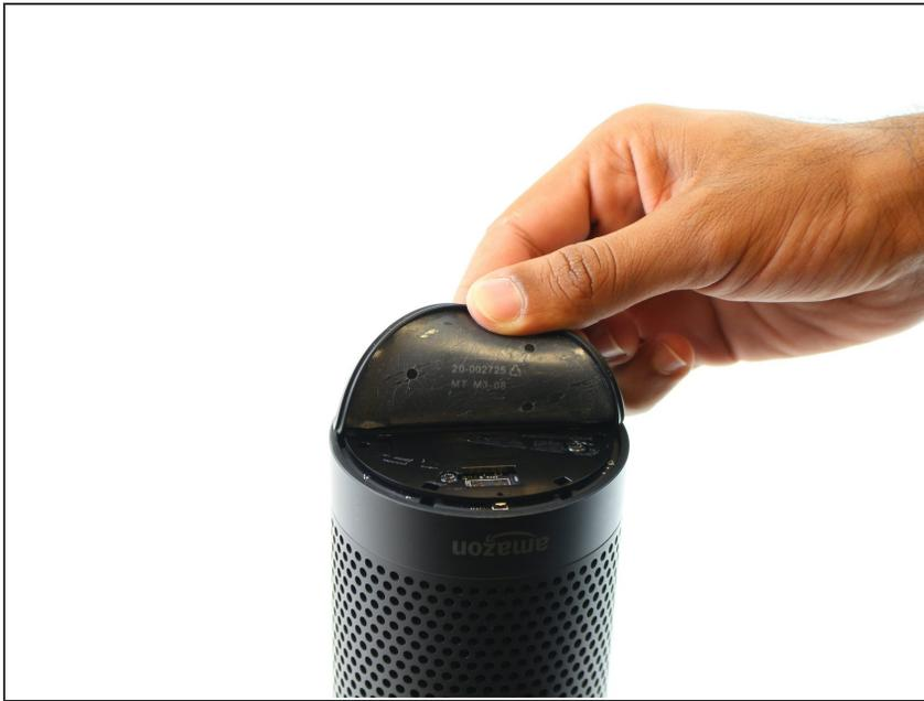
**⚠** Power off and unplug your Echo before disassembly. Failure to do so could result in injury or damage to the device.
