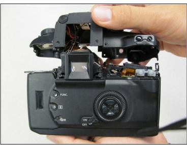
Slowly separate the top panel from the camera by pushing it upward.
