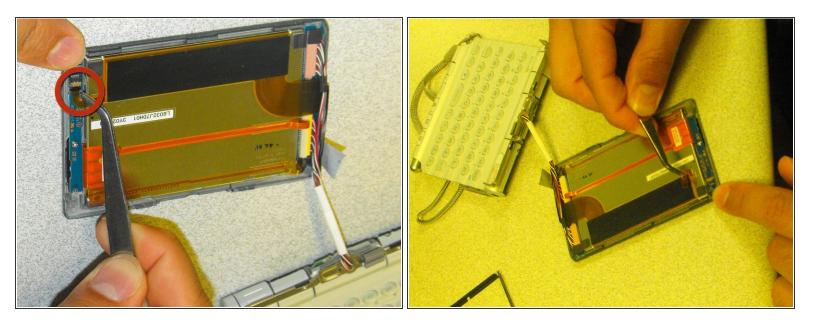
Disconnect the thin USB cable attached to the Integrated Circuit.
