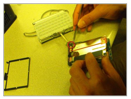
• Disconnect the thin connector from the face plate using tweezers.
