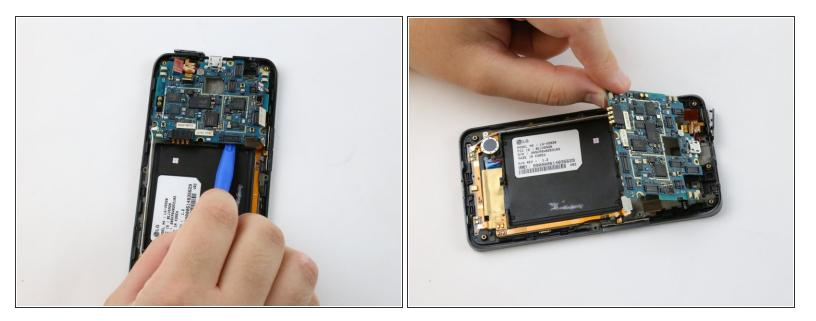
• Hook the plastic opening tool underneath the motherboard and firmly lift it out of the phone casing.
