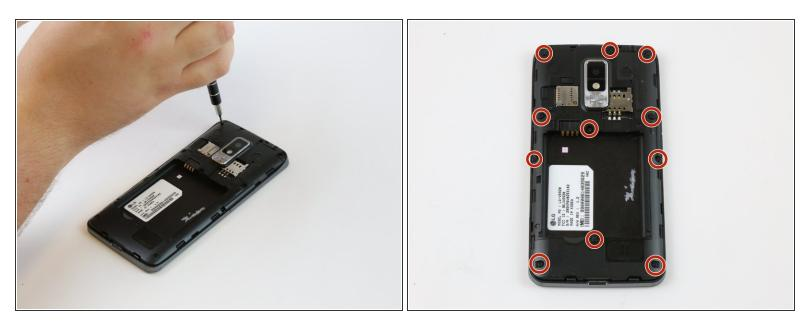
• Remove eleven 4mm Phillips #000 screws with a PH000 screwdriver.
