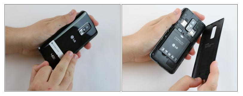
• Using your thumbnail, lift up on the notch in the middle of the bottom side of the phone.
