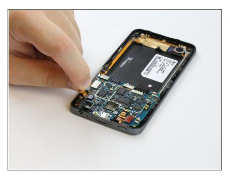
Remove the audio port from the motherboard with either your hand or the plastic opening tool.
