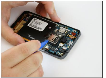
Hook the plastic opening tool underneath the plate and gently lift it up.
