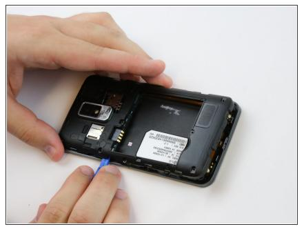
• Use the plastic opening tool to firmly pry up the plastic backing around the perimeter of the phone.
