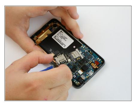
• Gently wiggle the plate side-to-side while pulling up to release it from the metal clamps holding it in.
