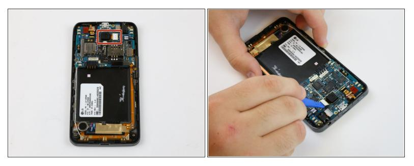
Use the plastic opening tool to lift up the connector that holds the camera to the board.
