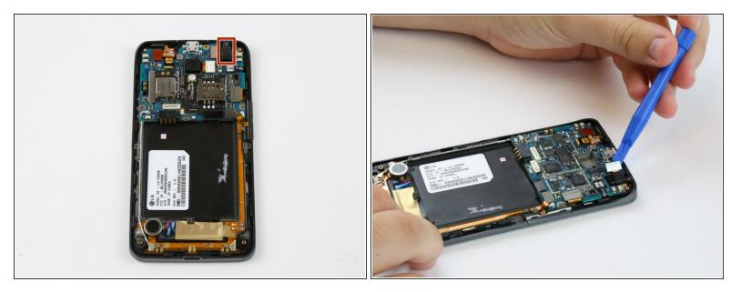
• Using the plastic opening tool, gently pry up the audio port connector.
