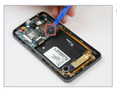
Detach the black rectangular film attached to the SIM/SD card plate with a plastic opening tool.
