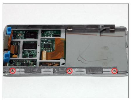
Remove the three Phillips screws securing the front panel to the metal framework.
