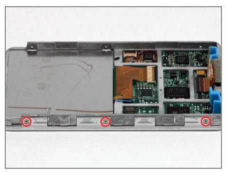
Rotate the iPod 180 degrees and remove the three Phillips screws securing the front panel to the metal framework on the other side.
