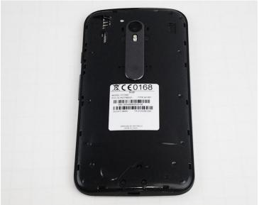
• Use your fingernail to pry under the notch on the bottom of the phone and remove the back cover.
