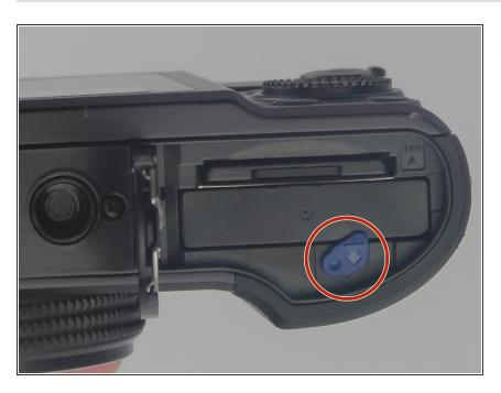
Push the blue button down in a clockwise motion and pull out battery.
