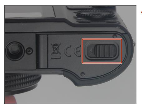
Slide battery lock in the direction of the arrow.
