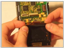
• Located near the bottom of the motherboard will be two ZIF connector tabs. Gently lift up the flap that secures these tabs and remove the tabs.
