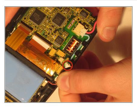
Screen-side down, unhook the battery cable from the motherboard.
