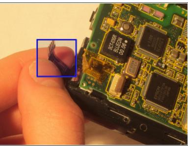
On the back of the motherboard near the top, gently lift up the flap that holds the ZIF connector tab
