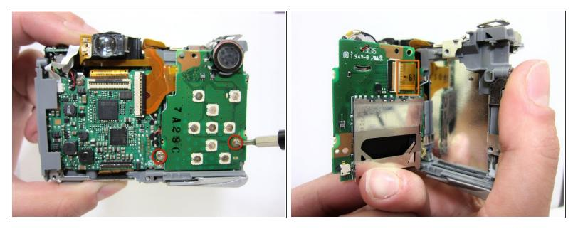
Unscrew 2 3.35mm phillips head screws from the face of the green circuit board using a #00 phillips head screwdriver.
