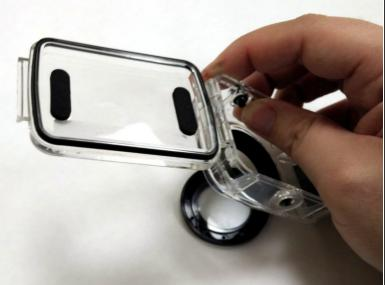
Apply pressure to the lens cover with your thumb, and use your other fingers to pull up on the case, separating the lens and lens trim from the case.
