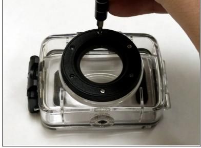
• Remove the six 4.5mm Phillips #00 screws from the black lens cover trim.
