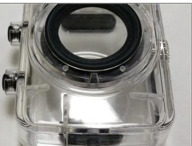
There is a small plastic key on the black bezel that aligns it to the case. Be sure to line this up during reassembly.
