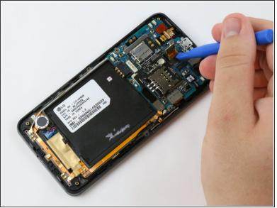
Remove the camera by gently lifting the film that is attached to it from motherboard with the plastic opening tool.
