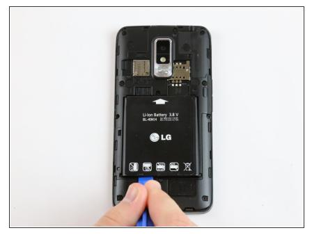
Using either your thumbnail or a plastic opening tool, lift up on the battery using the notch in the bottom left hand corner of the battery and remove it from the phone.
