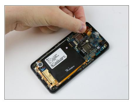
Use the plastic opening tool, or your hand, to pull up on the camera and remove it from the motherboard.
