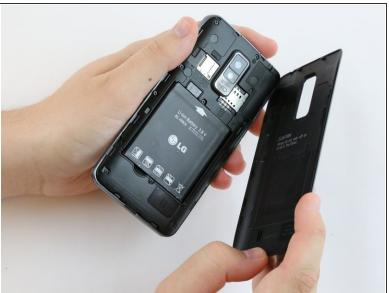
Using your thumbnail, lift up on the notch in the middle of the bottom side of the phone.
