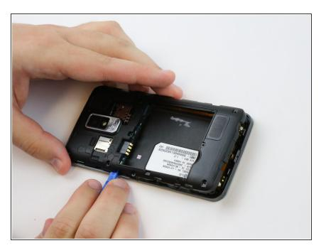
Use the plastic opening tool to firmly pry up the plastic backing around the perimeter of the phone.
