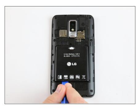
Using either your thumbnail or a plastic opening tool, lift up on the battery using the notch in the bottom left hand corner of the battery and remove it from the phone.
