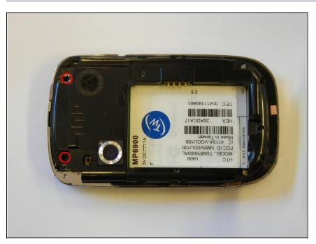
Remove the 2 torx-head screws located at the top corners of the phone using the T5 Torx Screwdriver.
