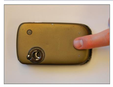
Remove the back panel by sliding up.
