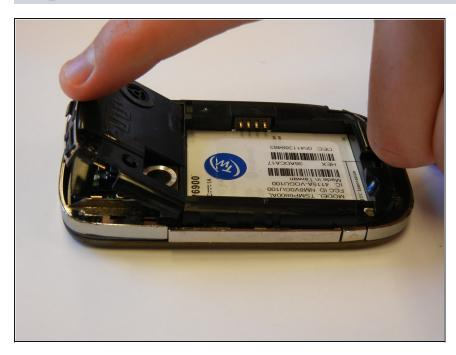
• Remove the plastic speaker casing above the battery slot.
