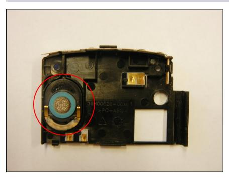
Use the plastic opening tool to remove the speaker.
