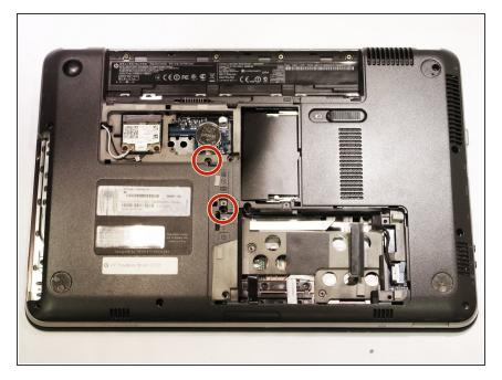
Remove 2 Phillips M2.5X6.5 screws from the back of the computer.
