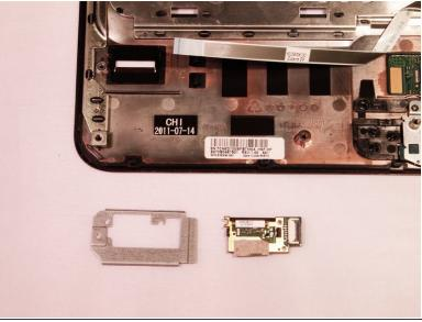
Release ZIF connector on fingerprint reader and remove fingerprint reader board.
