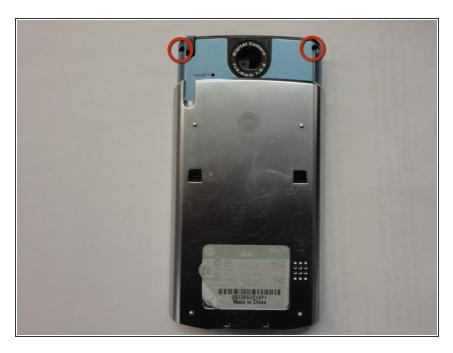
Use a Torx T5 screwdriver to remove the top two screws.
