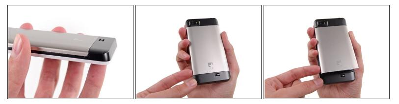
(i) There is a small indentation in the side of the phone near the bottom of the back cover.
