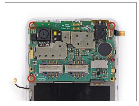
Remove the three 2.5 mm Phillips #000 screws securing the motherboard to the display assembly.
