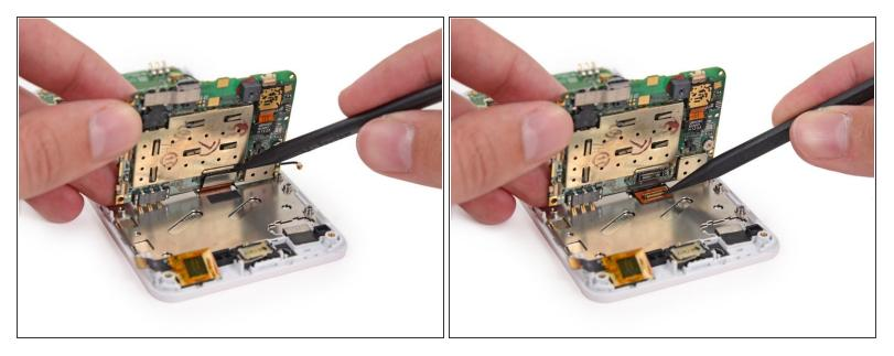
• Use the tip of a spudger to disconnect the display data cable from the back of the motherboard.
