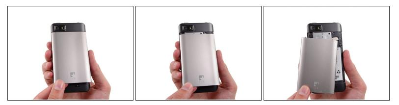
• Slide the back cover down and remove it from the phone.
