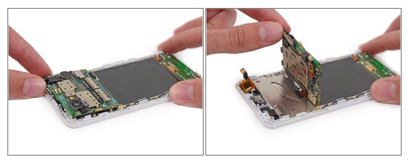
▲ Do not try to remove the motherboard just yet, as it is still connected to the display assembly by the display data cable.
