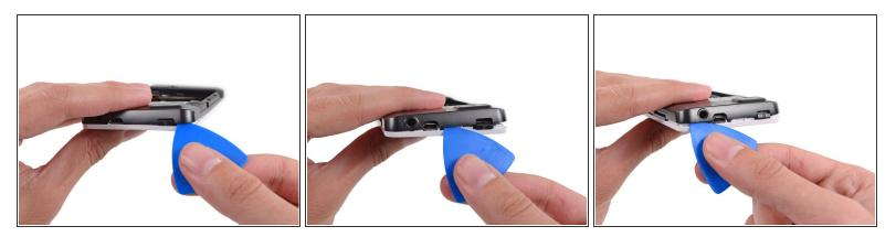
• Run the opening pick and pry along the top seam.
