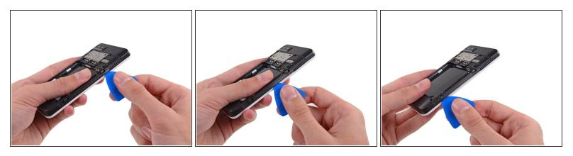
(i) The midframe is secured to the display assembly by several small plastic clips.
