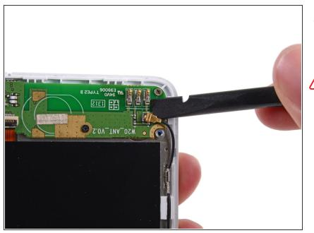
Use the flat end of a spudger to disconnect the antenna cable connector.
