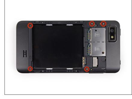
Remove the five 3.9 mm Phillips #000 screws securing the midframe to the display assembly.
