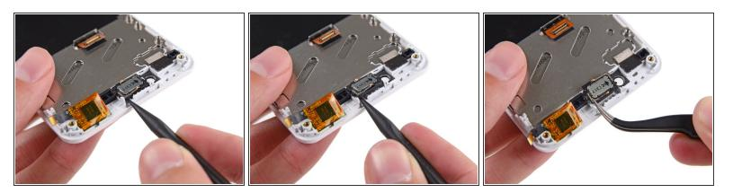
(i) The earpiece speaker is held to the back of the display assembly with some mild adhesive.
