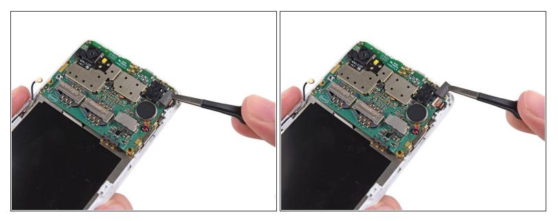
• Use tweezers to remove the adhesive foam tape from the top of the digitizer cable ZIF socket.
