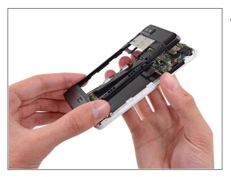
Separate any remaining clips and remove the midframe from the phone.
