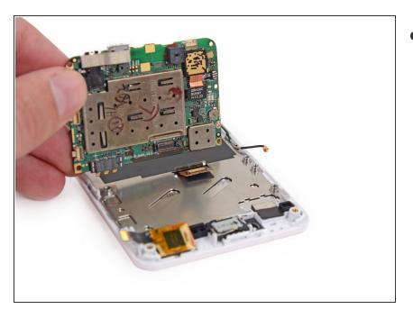
Remove the motherboard from the display assembly.
