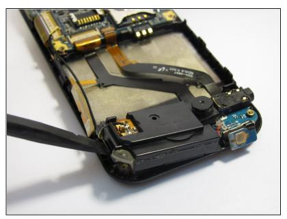
Pry the antennae/speaker component out of its casing.
