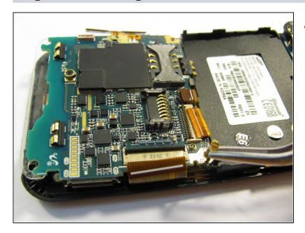
Pop the antenna plug off of its socket with a pair of metal tweezers.
