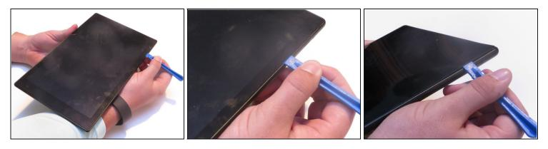
⚠ Avoid prying near bottom right hand side due to LCD Connector
