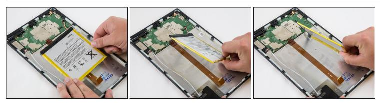
⚠ Make sure all the adhesive is removed before trying to lift the battery from the case.
