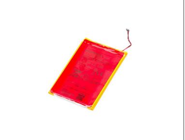
Use spudger to cut adhesive and pry the battery up.
