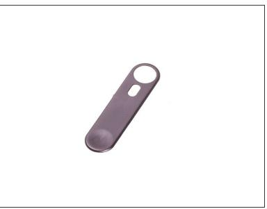
Remove camera&flashlight metal cover. Use tweezers to cut strong adhesives underneath.
