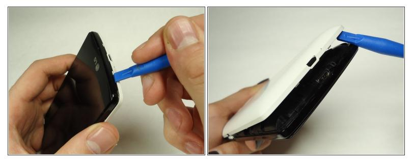
• Use the plastic opening tool to pry off the back cover.
