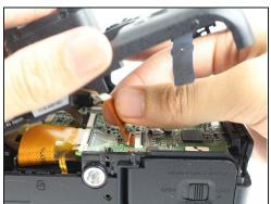
⚠ Do not yank off the back plate. If you do, you will tear the electronic ribbons attached to the inside of the camera and the back plate.
