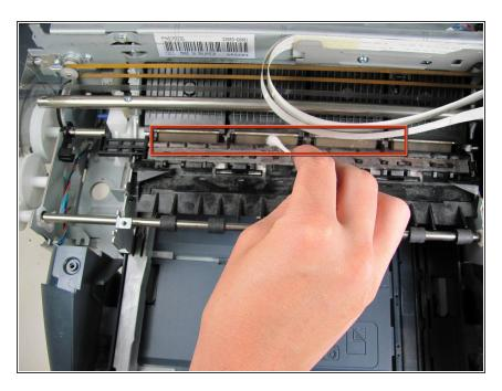
While rotating the feed rollers, clean them with purified or distilled water and a lint-free cloth.
