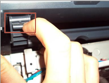
Press down on the two plastic hinges to remove the upper portion of printer.
