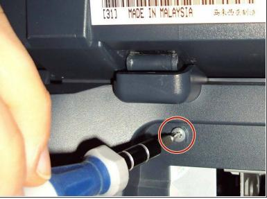
Using the T10 Torx Security Bit Screwdriver, unscrew the screws on the upper left and right corners of the inner panel to remove the inner back panel.
