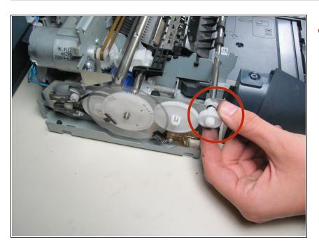
Turn the smallest white plastic gear on the left side of the printer to rotate feed rollers.
