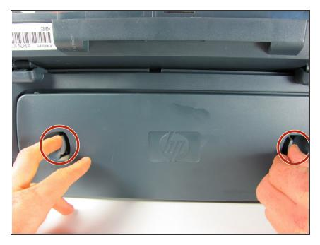
Remove the back panel by inserting your fingers into the indentations next to the tabs. Press the tabs inward towards each other while pulling the back panel toward you.
