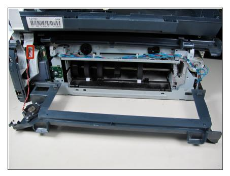
Grasp the plastic plug on the end of the speaker wire, then gently pull the plug away from the printer until the wire is removed.
