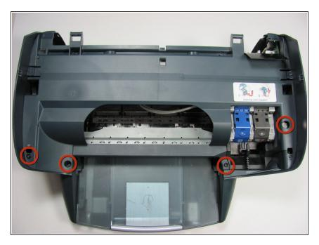
Using the T10 Torx Security Bit Screwdriver, remove the four black screws holding the printer carriage cover in place.
