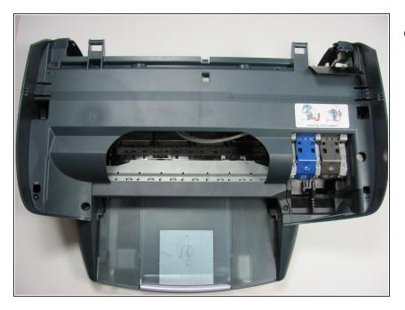
Detach the scanner tray from the printer by lifting the scanner tray off the printer body.
