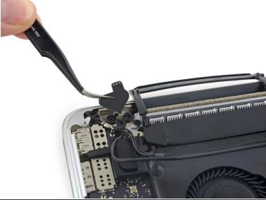
Remove the two rubber hinge covers.
