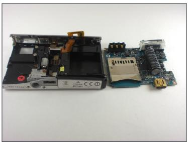
• lift motherboard from the top to remove it from the camera.
