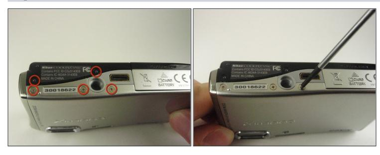
• Remove all five screws from the bottom of the camera using a Phillips #00 screwdriver.
