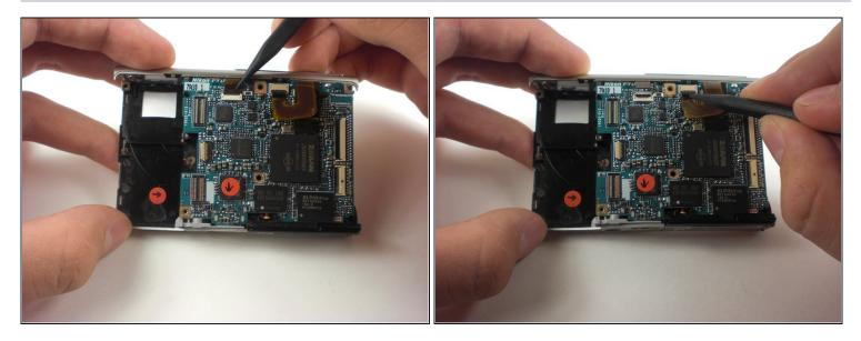
• Lift two flaps with the spudger on the top of the motherboard to release ribbons.
