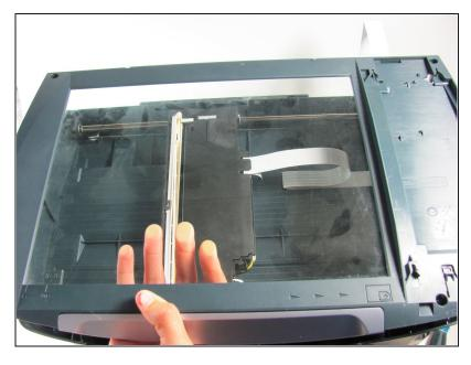
Once you have removed the four torx screws, gently lift the scanner glass cover from the printer's base.
