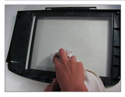
Moisten a lint-free cloth with alcohol. Wipe down the underside of the scanner glass until all dust is removed.
