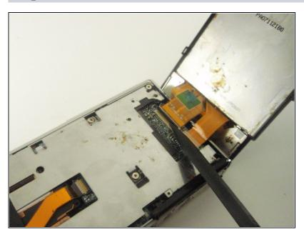
With the back cover lifted, lift the black flap that connects the ribbon to the motherboard with the spudger and carefully remove the back cover.
