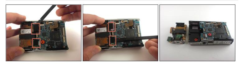
• Lift the two ribbons with the spudger to disconnect the lens and pull it out.
