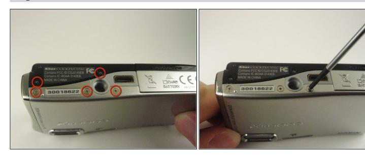
• Remove all five screws from the bottom of the camera using a Phillips #00 screwdriver.
