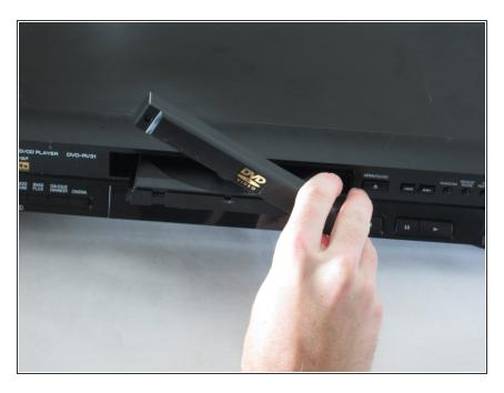
Evenly lift upward on the disk tray front cover (not slanted, as pictured).
